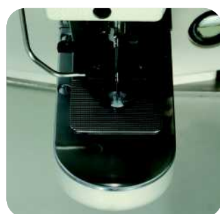
Equipped with the thread column device for whipping (Column height: 2-10mm)
